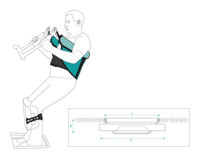
The Staebel Standing Loop Sling is for use with the stand up hoists with loop attachment. It features optimum back support and under arm padding for a safe and comfortable lift and also allows for the easy removal of clothing for toilet transfers. It features a torso band for security and stability with Buckle (272TL03) or Velcro fastening (272TL04).
